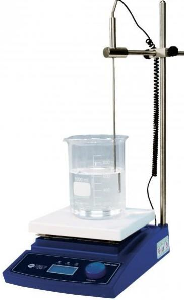
A photograph of a magnetic stirrer. It features a blue base with a digital control panel and a white heating plate. A clear glass beaker is placed on the plate, containing a light-colored liquid. A magnetic stirrer bar is submerged in the liquid, connected by a black cord to a vertical metal post. The post has a coiled black cable attached to its top. |
